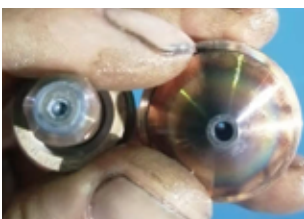
260A 20 mm plate cutting After 200 times pierce 300 meters cutting Almost no loss
