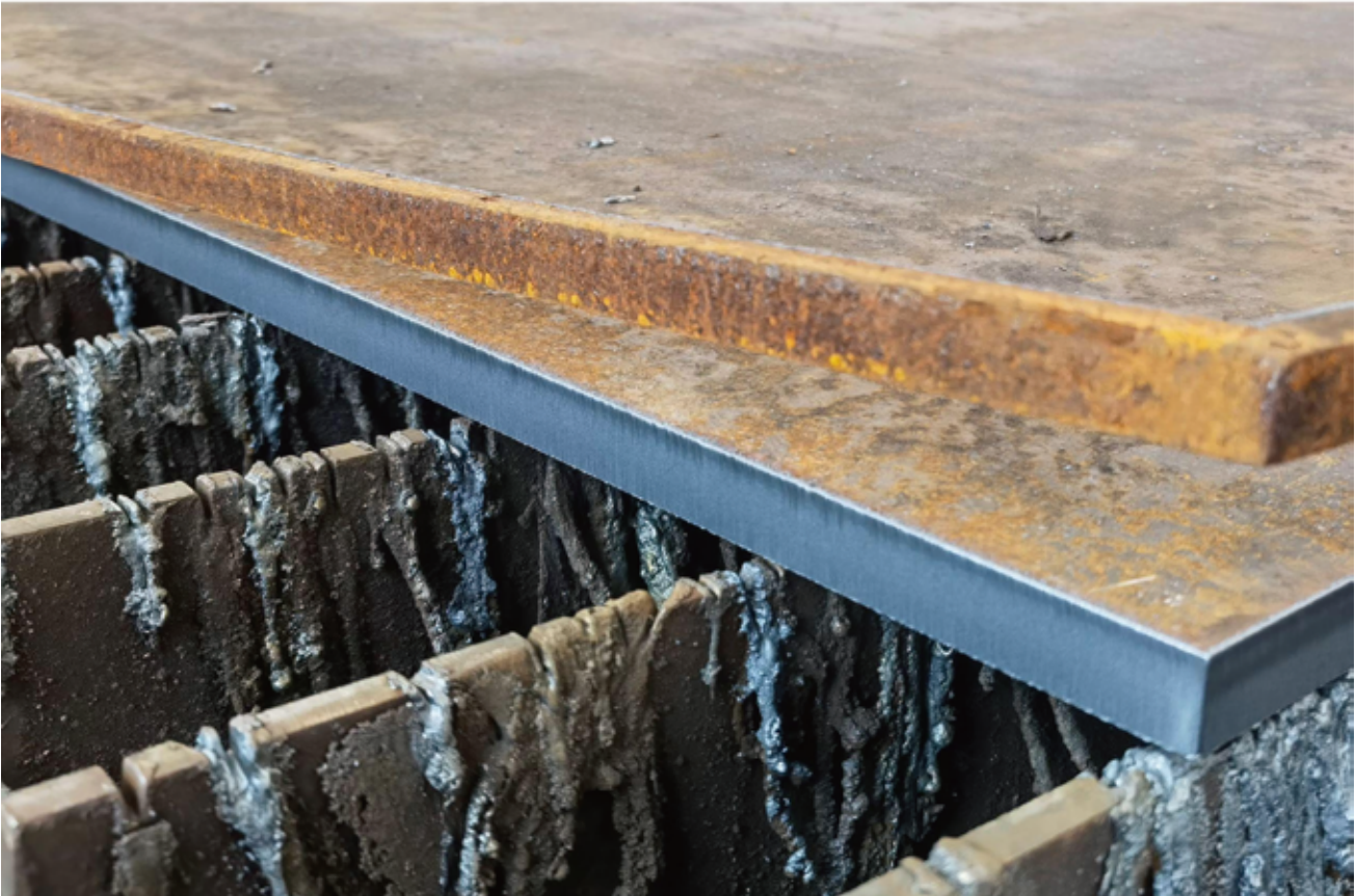
MS 20 mm, Oxygen/Air, Speed 1200 mm/min, by MAX130
