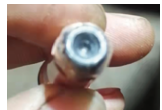
260A 20 mm plate cutting After more than 800 times Pierce 700 meters cutting Total run out
